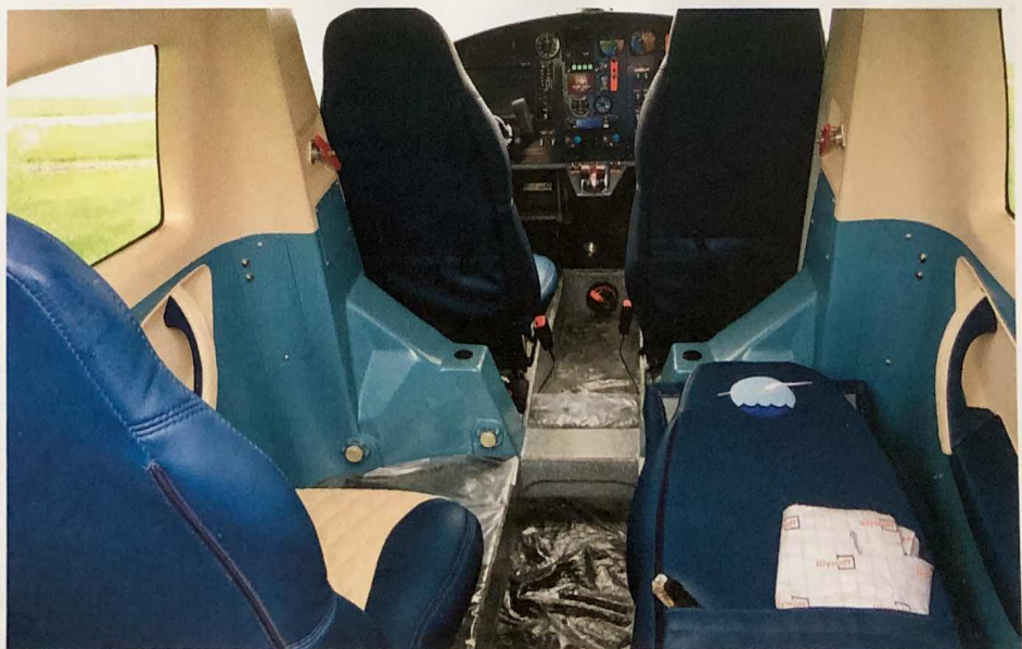
L44 cockpit (above) is a modern, spacious environment, as is the passenger cabin (below). The seats fold forward for easy cockpit entry and egress, and for carrying bulky cargo.
